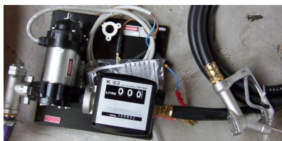
Flow meter & Fuel transfer pump
